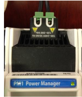
PM1 top view - 100~240VAC input terminals
