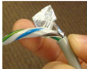
Figure 2: To minimize emissions with the optional PM1 Power Supply module, optionally use a shielded power conductor.
