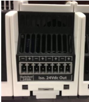
PM2 front view – 24VDC output terminals
