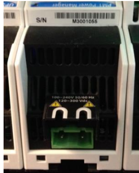
PM1/PM2 rear view - 100~240VAC input terminals
