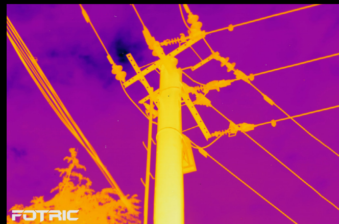
1280*1024 IR resolution (25° lens at 30m distance)
