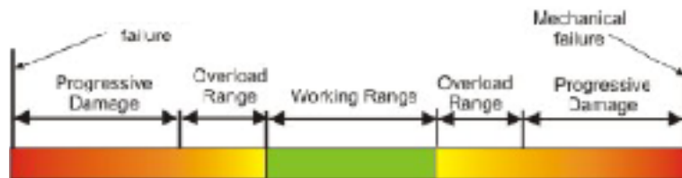
Load ranges for a typical load cell
